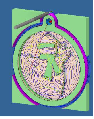
I really want four of these. Running these separate would require several tool changes for each part. I would rather run all four at once. That can be done with a Pattern.
